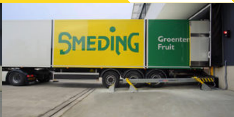
Multiple axle and rear-steering axles trailers.
