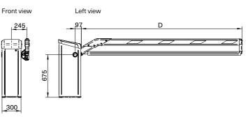
are available as left and right versions. If one looks at the barrier housing down the boom from its tip, the boom is on the left in the L variant and on the right with the R variant.
