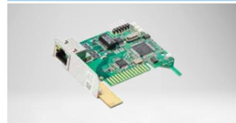
> Extension modules for easy control of barriers via Ethernet, RS-485, radio (433 MHz) or mobile communication (GSM) > Counting modules for networking barriers and recording the incoming and outgoing vehicles
