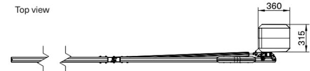
All barriers from Magnetic are available as left and right versions. If one looks at the barrier housing down the boom from its tip, the boom is on the left in the L variant and on the right with the R variant.
