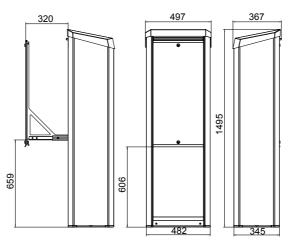
Terminal-MXL Side view with fully extended front panel, from the front and from the opposite side
