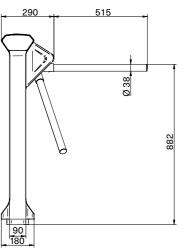
Mounting space for reading devices for mTripod and mTripod short (without passage indicator, mounting depth 40 mm)
