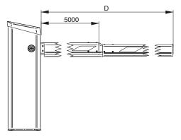
All barriers from Magnetic are available as left and right versions. If one looks at the barrier housing down the boom from its tip, the boom is on the left in the L variant and on the right with the R variant.
