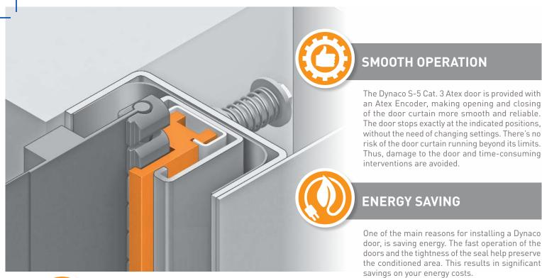
an Atex Encoder, making opening and closing of the door curtain more smooth and reliable. The door stops exactly at the indicated positions, without the need of changing settings. There's no risk of the door curtain running beyond its limits. Thus, damage to the door and time-consuming
